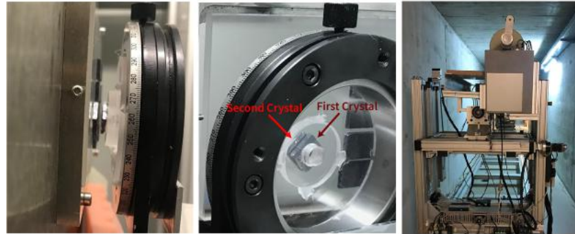
Figure 4.11: Experimental configuration of the two coupled crystals. Left photo : side view of the crystals. The quartz frame on which one of the two crystals is glued is the sheet on the left side, while on the right side one can see the rotatable sample holder with the adjustable crystal. Center photo : front view of the coupled crystals. Right photo : the imager detector and the spectrometer used in our experiment.
