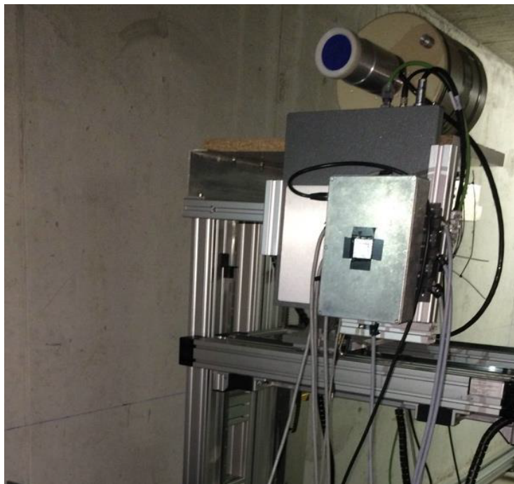
Fig 10: The Compton-POLCA detector, mounted in place of the LARIX-T imager (gray box).
