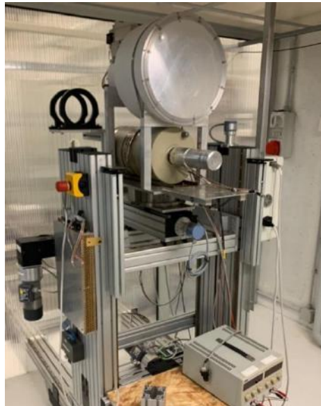
Figure 10: Picture of the Detectors holder carriage with the imager on top and spectrometer on bottom.
