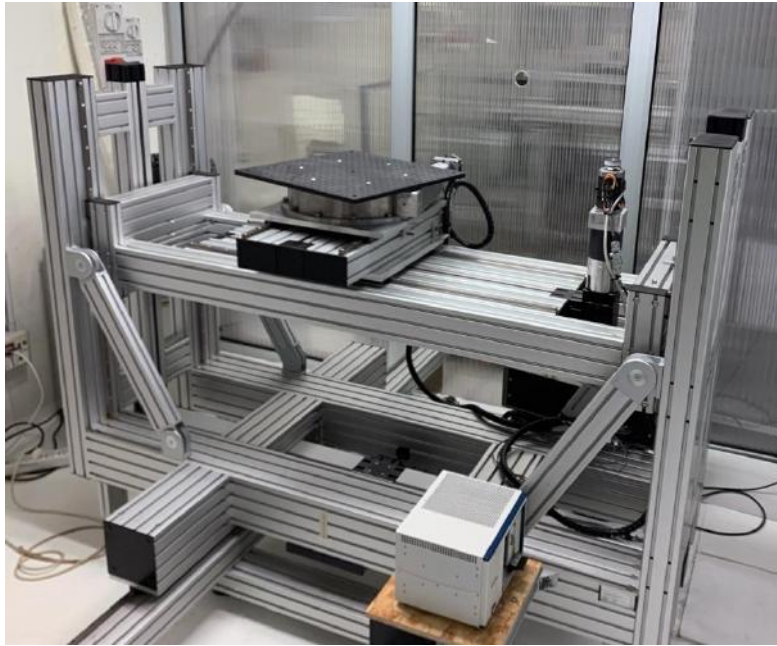
Figure 8: Picture of the sample holder.
