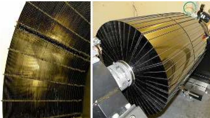
Figure 1.9: The image showing 133 nested cylindrical mirror shells of one of the two optical units onboard NuSTAR.
