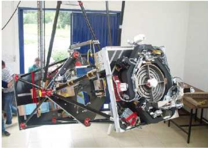
Figure 1.10: The CLAIRE telescope at the Gap–Tallard balloon base during the 2001 balloon campaign. On the first platform, the gamma-ray lens in its two-axes gimbal. [34]
