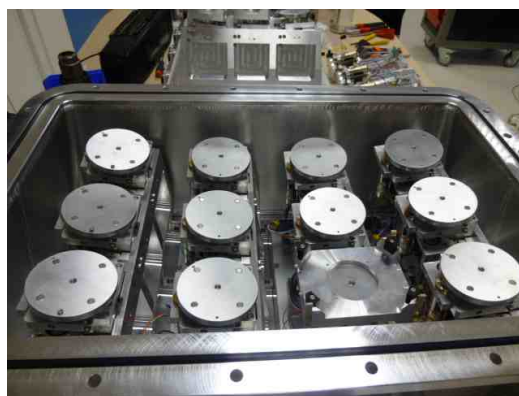
Figure A.7: Picture of the unit for the housing of 12 analyzer crystals.
