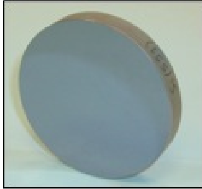
Figure A.9: An anodic bonded elastically bent analyzer.
