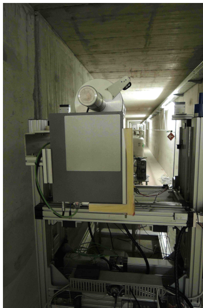
Figure 7.10: The focal plane detectors used in the LAUE project: the flat panel detector is positioned below the HPGe detector.
