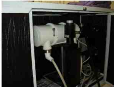
Figure 5.2: A view of the X-ray generator tube, located in a lead box.
