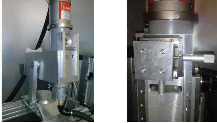
Figure 7.4: Left : The X-ray source that is being used for assembling and testing the lens petal. Right : A detail showing the 1 mm lead collimator placed in front of the X-ray tube aperture.
