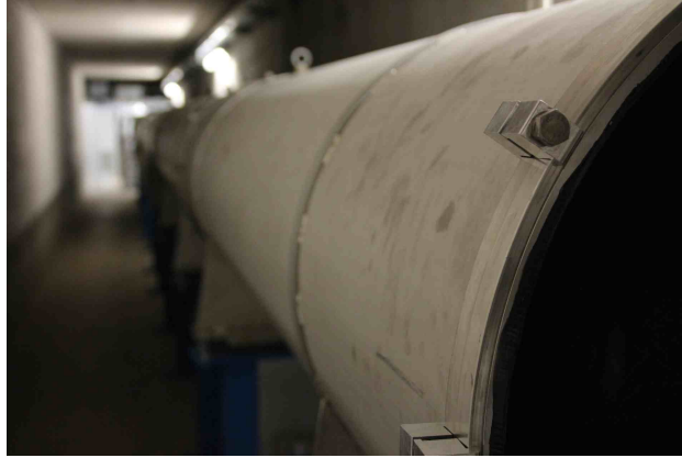
Figure 7.5: The 21 m beam line in which is carried out the vacuum for avoiding absorption and scattering.
